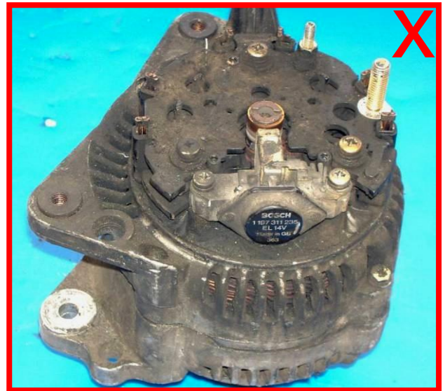
Missing plastic cup → not acceptable
